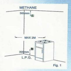
The Domestic detector should be wall mounted near to any source of gas such as a cooker. When a heavier than air gas is being used then the detector should be mounted approximately 300 mm from the floor and within 2 metres from the gas source. For lighter than air gases such as methane then the detector should be 300 mm from the ceiling. See Fig. 1
