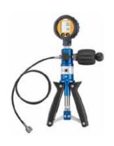
SIKA Precision Pressure Calibrator Type PM 700 P Pressure medium-distilled water or hydraulic oil Measuring ranges 0....500,0...700 bar Display multi-purpose LCD,20 X 60 mm Switchable pressure units bar,mbar,PSI,kPa,MPa
