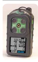
The Solaris Multigas Detector is an economical, 4-gas instrument providing simultaneous detection of CO, O2, H2S and combustible gas. It weighs less than 8 ounces, and has an IP 6/5 rating against liquid and dust ingress. The Solaris Multigas Detector is powered with a rechargeable lithium ion battery that offers 14+ hours of continuous run time and fully recharges in less than 4 hours. Calibration is intuitive and is accomplished with the push of a single button.
