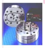
SIKA positive displacement flow sensors are highly accurate transmitters that measure volume flows. They work on the positive displacement principle. The flowing medium causes a pair of gear wheels to rotate. The sensor is manufactured to the highest accuracy and is then precisely assembled. The rotation is scanned by two non-contact pick-offs.
